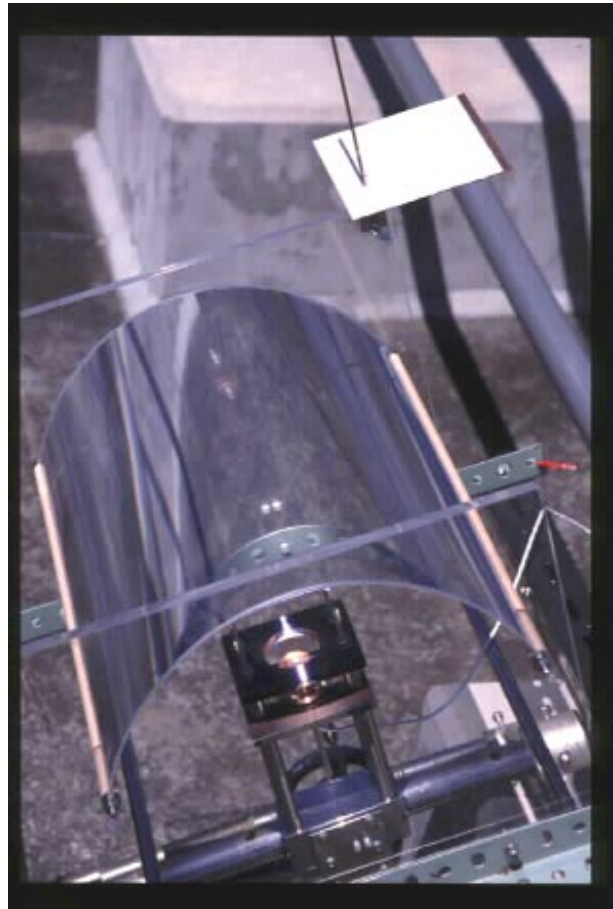
Figure 6: Experimental setup to measure the radiation flux distribution of a linear nonimaging Fresnel lens with acceptance half angle pairs of \pm\theta = 2^\circ , and \pm\psi = 12^\circ . The lens is intended as solar concentrator for photovoltaic applications. Lens length is 400 mm. 30 July 1999, Tokyo, Japan.
