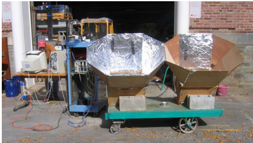
FIGURE 1. PARAMETRIC TESTING SETUP OF BOX COOKERS.
