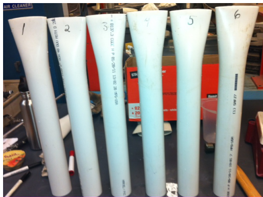
Figure 9: Pipes molded using the metal mold
