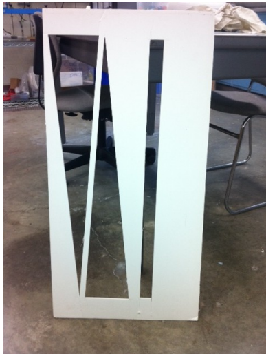
Figure 4: Cut outs of mold sides for plaster form
