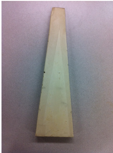
Figure 3: Mold for 3" pipe made out of plaster of paris and coated with polyurethane
