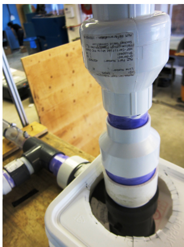
Figure 3: Waste valve and waste collection bucket detail.
