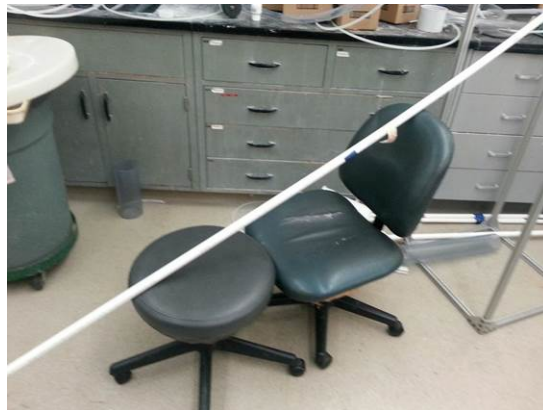
Figure 7: Make-shift stabilization system for drive pipe
