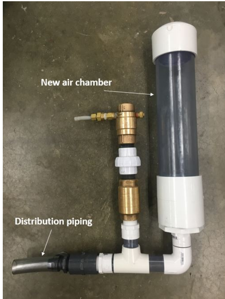
Figure 11: A second air chamber was installed next to the ram pump exit and behind the distribution piping in order to eliminate the vacuum effect. (Galantino et al., 2016)
