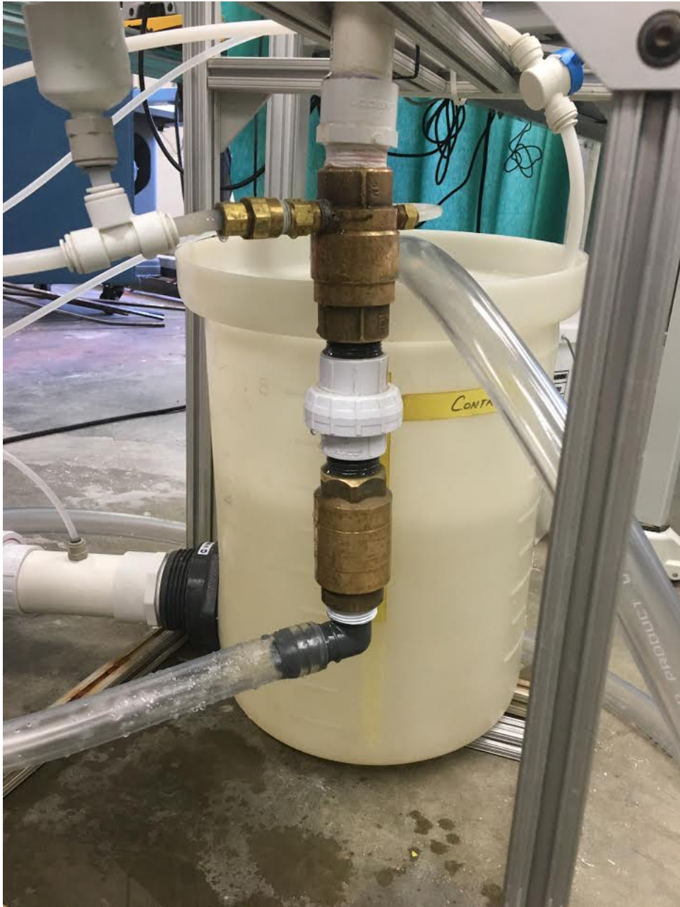
Figure 10: In order to simulate a completely submerged ram pump, distribution piping was added to the bottom of the apparatus using flexible plastic tubing and a barbed adapter fitting. (Galantino et al., 2016)
