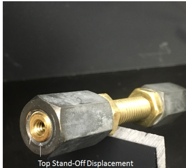
Figure 15: This shows the top standoff in its zeroed position. Positive displacement occurs as it travels further down the threaded portion of the rod.
