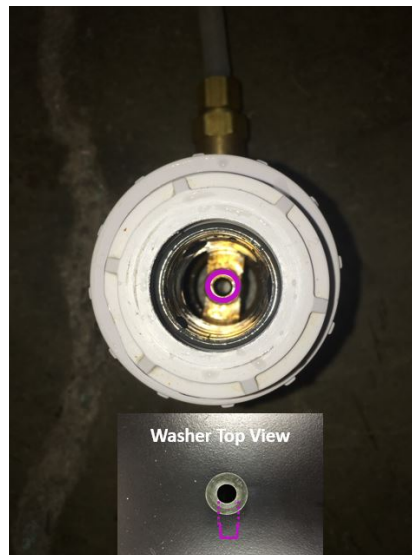
(b) A washer was added between the check valve and the problematic collar, to prevent the pump from jamming. Note that the diameter of the washer's opening is smaller than that of the collar, to effectively screen the edge of the collar from the check valve.
