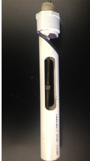
(a) This is the unenclosed PVC prototype of the ram pump.
