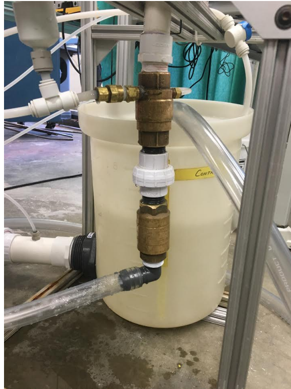
Figure 17: In order to simulate a completely submerged ram pump, distribution piping was added to the bottom of the apparatus using flexible plastic tubing and a barbed adapter fitting.
