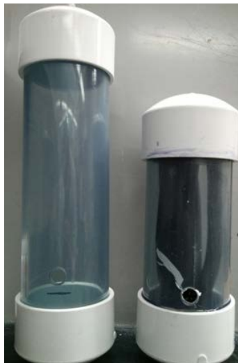
Figure 8: Two of the different air chambers available - 15 inch (L) and 12 inch (R).
