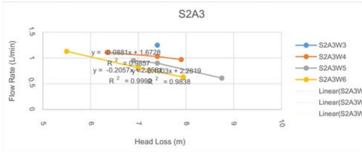
Figure 12: Relation between flow rate and head loss for different arrangements: “S#” stands for the number of the drive pipe system, “A#” is the number of air chamber and “W#” is the number of 50g weights.
