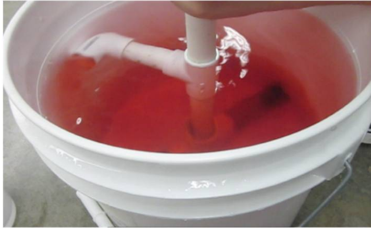
Figure 2: The centrifugal pump is able to lift the dense red sugar solution and discharge it near the surface of the tank. A movie of this is posted online.
