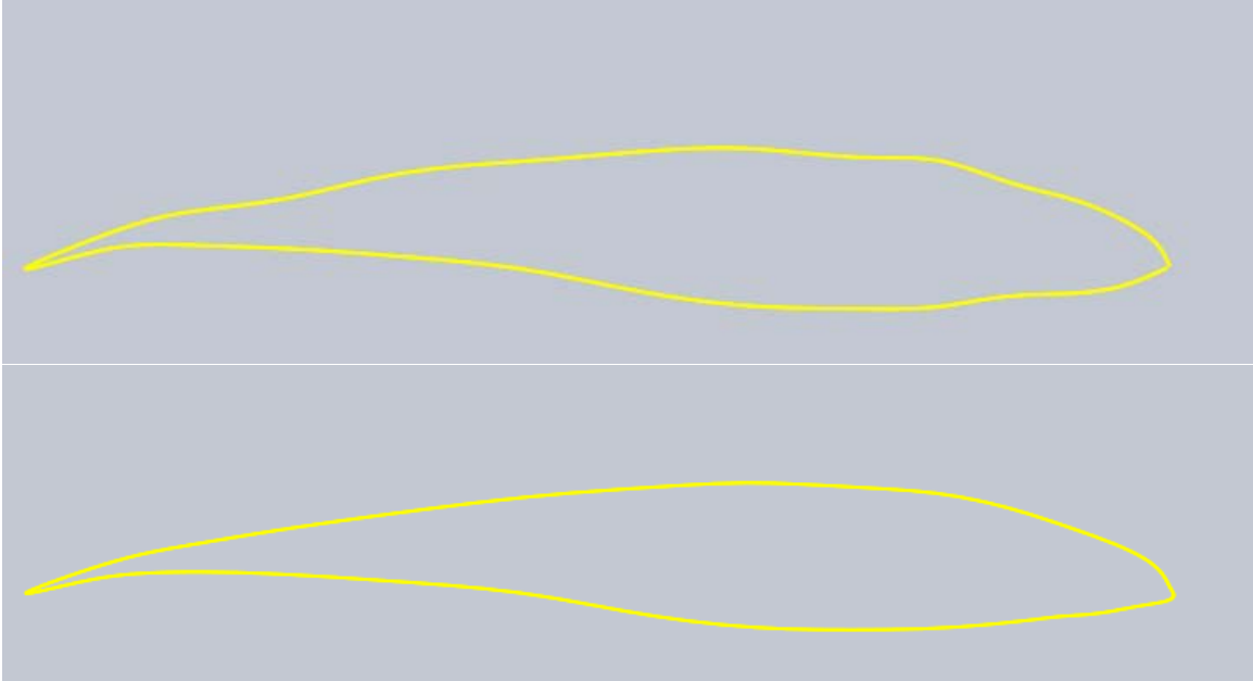
Figure 5: S826 Airfoil with Unmodified (top) and Modified (bottom) Point Data
