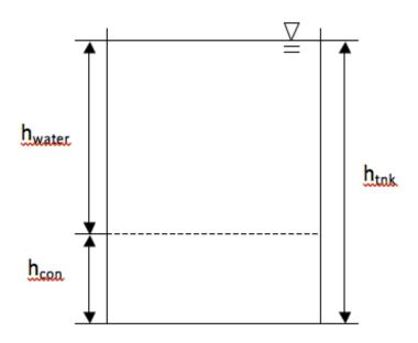
The potential energy of the concentrated salt layer ( $E_{saltSoln}$ ) is a function of the salt density ( $\rho_{concSoln}$ ), area of the tank ( $A_{Tank}$ ), the ratio of the concentrated solution volume and the total volume ( $r_{soln}$ ), the height of the tank ( $H_{Tank}$ ), and gravity (g) (Equation 1).
