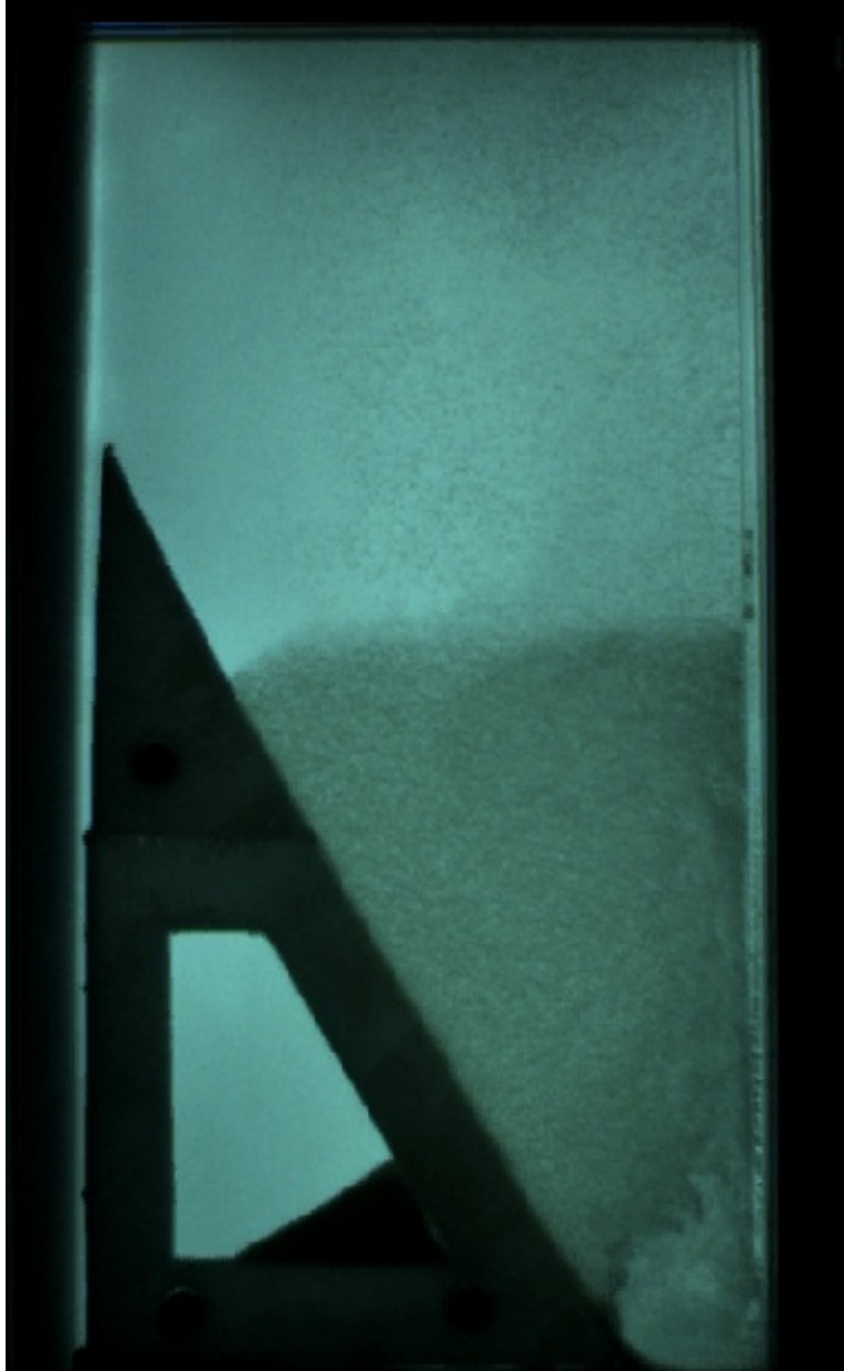
Figure 34: Floc blanket forms and slowly grows to the top of the insert
