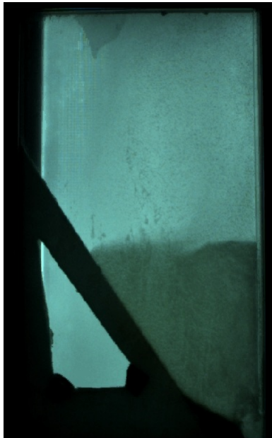
Figure 8: Floc blanket reforms after alum stock is replenished
