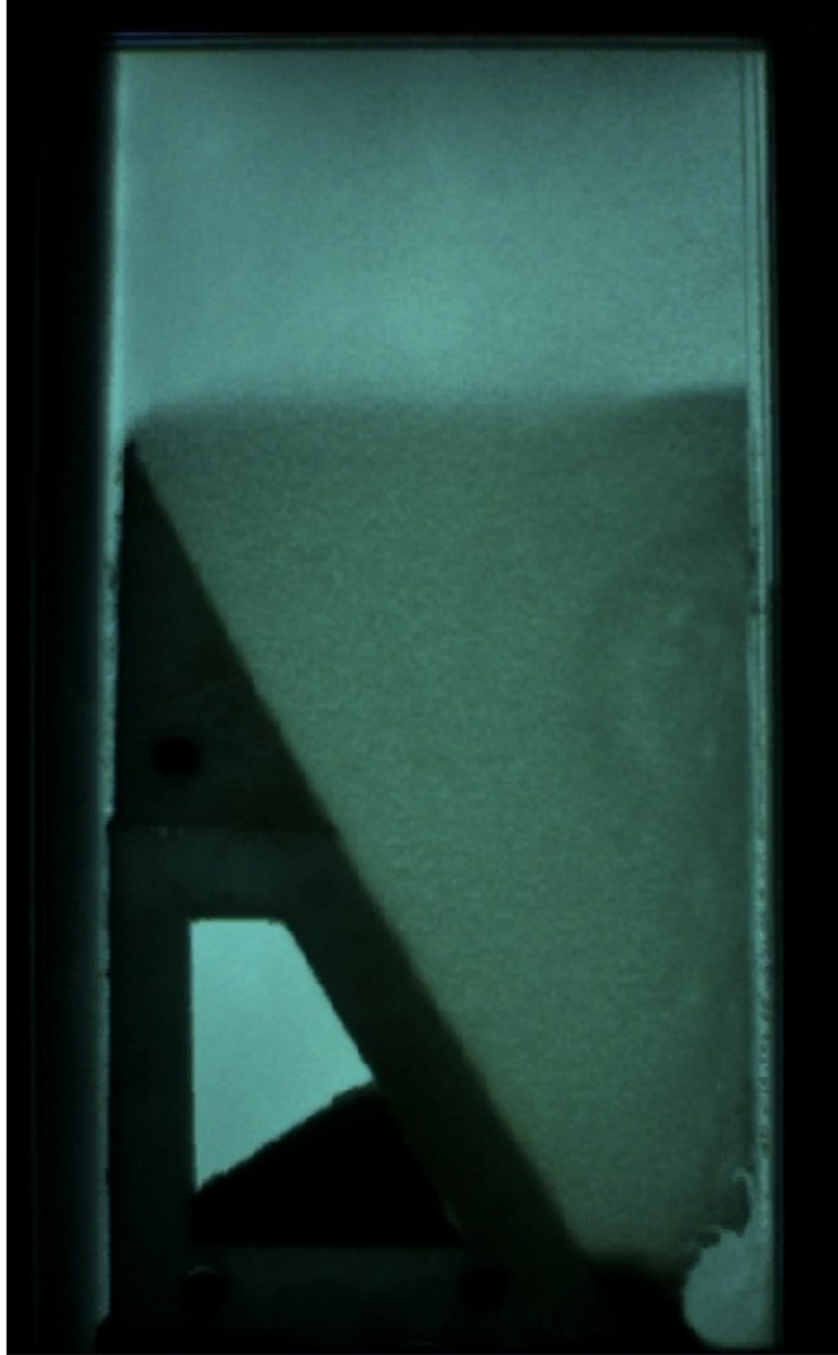
Figure 36: Sludge accumulates slowly in the hopper, but mass is not conserved due to flocs leaking into the hole within the insert
