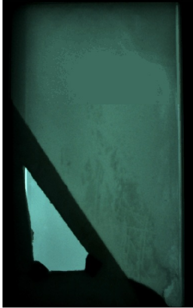
Figure 7: Floc blanket thins out after alum stock runs out
