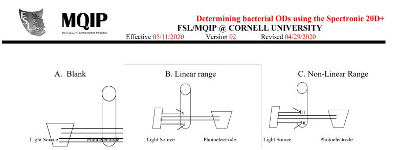
In the linear range, the amount of light transmitted to the photoelectrode is directly proportional to the amount of bacteria in the tube. However, if measurements are made outside the linear range, the relationship is no longer proportional and is inaccurate. This is due to the concept shown in figure c which demonstrates that the more bacteria that are in the tube, the more likely it is that a significant portion of the bacteria are not diffracting light.
