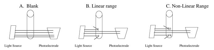
In the linear range, the amount of light transmitted to the photoelectrode is directly proportional to the amount of bacteria in the tube. However, if measurements are made outside the linear range, the relationship is no longer proportional and is inaccurate. This is due to the concept shown in figure c which demonstrates that the more bacteria that are in the tube, the more likely it is that a significant portion of the bacteria are not diffracting light.
