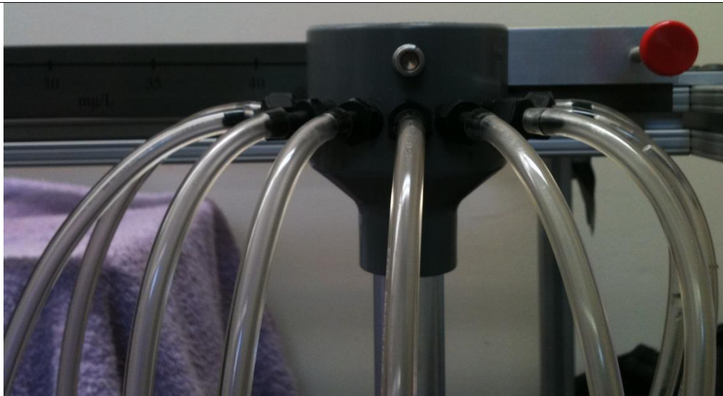
Figure 17: Image of reducer with 9 small diameter tubes attached
