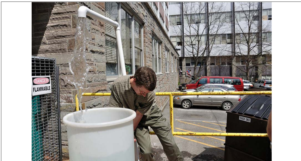
Figure 16: Team Leader Monroe Weber-Shirk testing Diaphragm Pump
