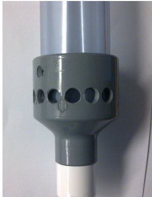
Figure 6: Coupling attached to the rotation rod.
