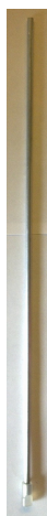
Figure 3: Working hydrometer design which includes 0.115 in diameter Aluminum tubing with a weight attached to the bottom.
