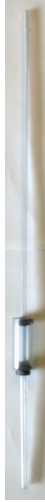
Figure 2: Second design using clear PVC. This design is a modification of the previous design to include a small chamber of air at the bottom of the hydrometer.
