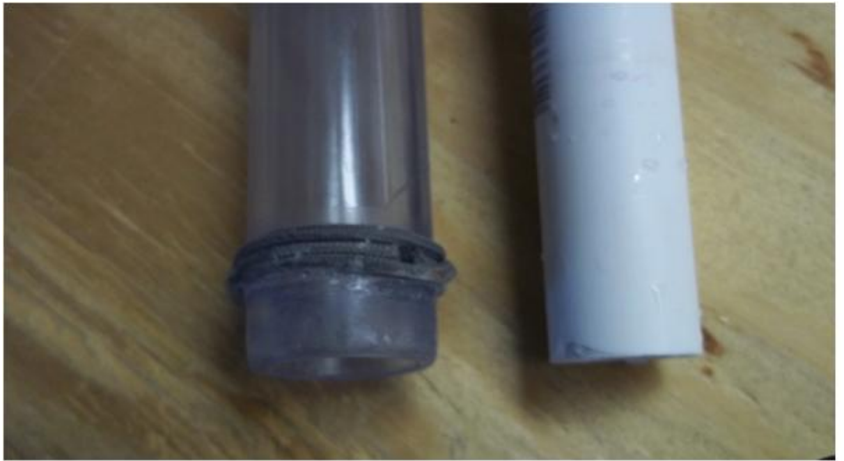
Figure 2: The tighter seal between the suction rod and the rotation rod (left) contributed to the improved efficiency of the new pump (right).
