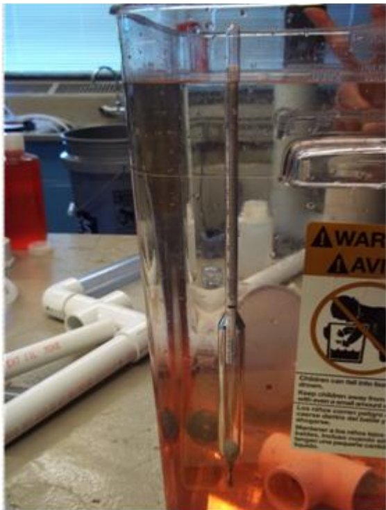
Figure 9: Obtaining measurements with the hydrometer.
