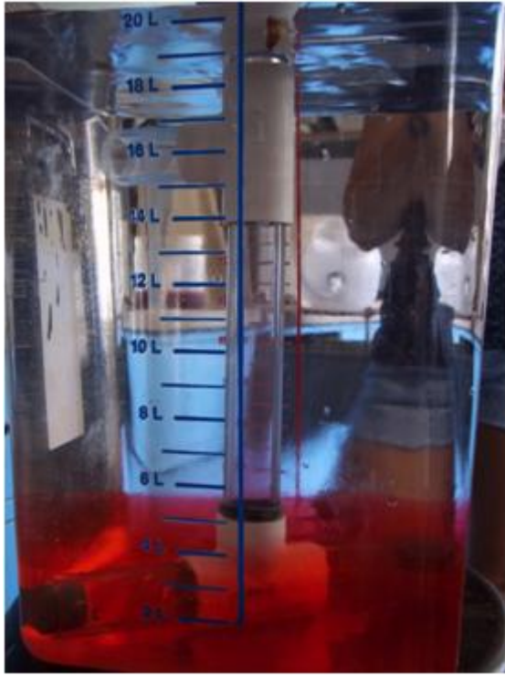
Figure 3: Improved centrifugal mixer assembled in a clear plastic 20 L tank with concentrated sugar solution at the bottom.
