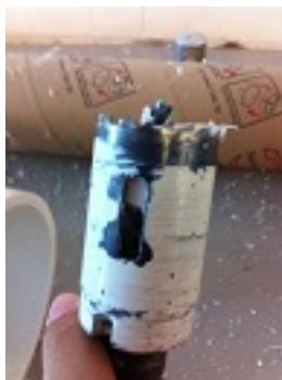
Figure 2.1: Vertical view of plug stuck in hole saw
