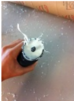
Figure 2.1: Vertical view of plug stuck in hole saw
