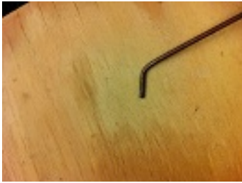
Figure 2.4: Bent prying end of tool
