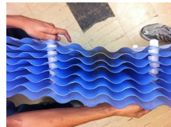
Figure 3.10: Cross-section view of complete plate settler module
