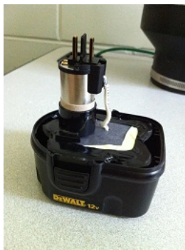
Figure 1.1: Disassembled Dewalt 12V Battery Pack
