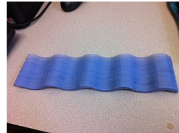
Figure 3.2: New Plate Settler Jig
