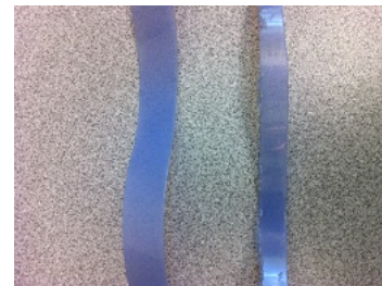
Figure 3.3: Comparison between scissors (left) and saw (right)
