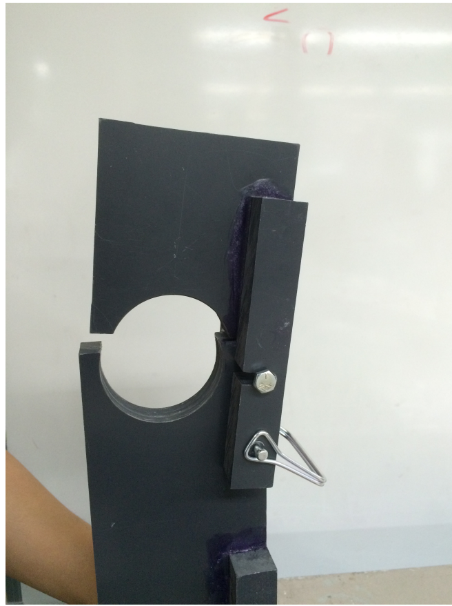
Figure 14: A close-up of the top spacer illustrating the degree of rotation exhibited even with a cotter pin installed.
