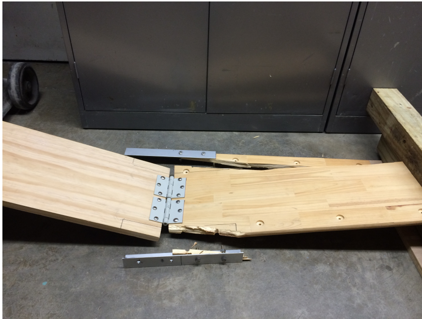
Figure 21: The full scale platform was broken when the team conducted stress testing on the scale. The highest observed force before failure occurred at 160 lbs.
