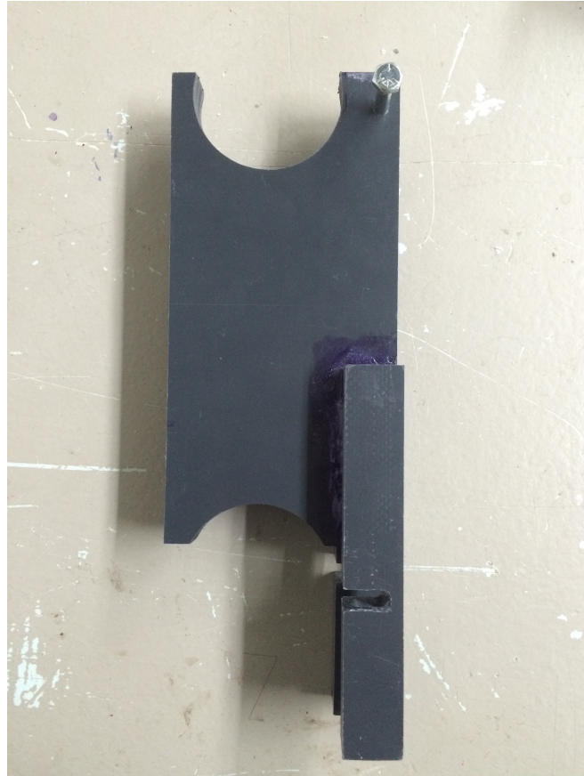
Figure 11: The completed fabrication of a middle spacer. The top right corner depicts the 1/4" bolt that will serve as a rod. The bottom right side of the spacer depicts latches with slots that will hold the rod of the spacer below. The cutouts are shown on the top and bottom of the spacer body. The cutouts are not symmetrical to allow for a greater degree of rotation of the spacers during installation.
