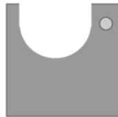
Figure 7: Schematic for the second design of the bottom spacer in front view. This design includes the rod in the upper right corner.
