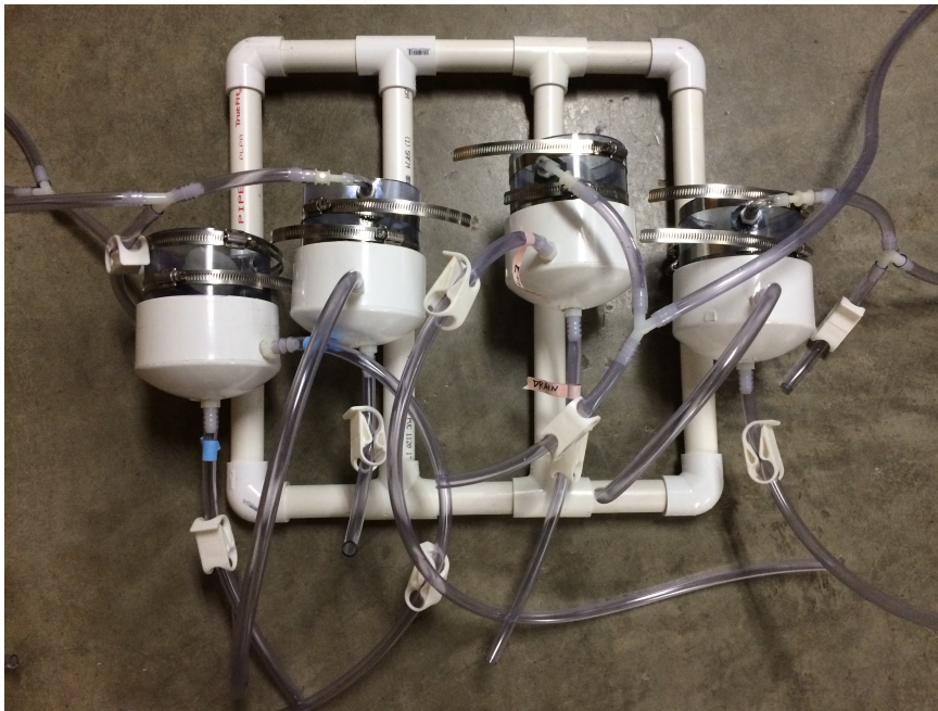
Figure 23: Schematic of the PVC Pipe Tank Design showing the mounting system of an individual CHT. The CHT is attached to a rectangular PVC bar using two large hose clamps. This PVC bar is secured to the 1" mounting pipe
