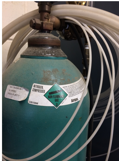
Figure 8: The compressed nitrogen tank that is the air supply for the plastic welder
