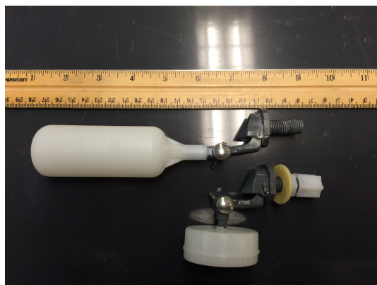
Figure 3: The float that originally comes with the float valve is shown on top and the custom made float is shown on the bottom. The first iteration of the CHT design accommodates the larger original float valve.
