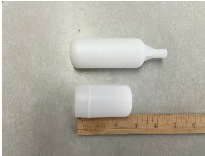
Figure 6: Comparison of the original 5 inch float that comes with the float valve shown on top and the spring 2015 CHT designs 2.5 inch float shown on the bottom.
