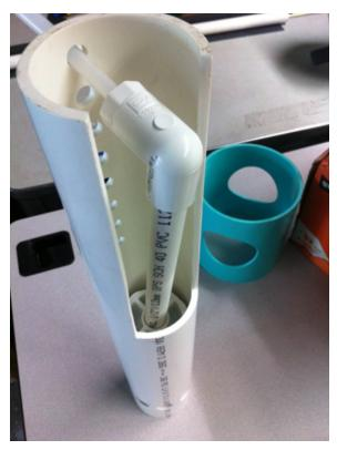
The float is locked into a certain height setting by the elbow piece which slots into one of the ½ holes. As the water level rises, the float will cause the whole vertical pipe to rise with it, throttling the flow. The ½ inch holes span 20cm, giving the operator multiple setting options for the float valve.
