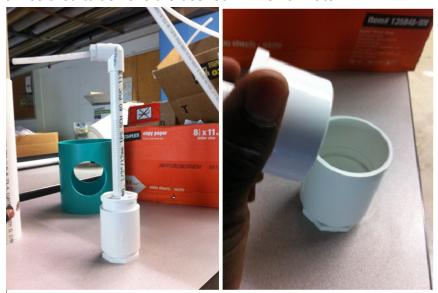
These pictures show the float, which is just a combination of a plug, coupling, and bushing, used to create a pocket of air.
