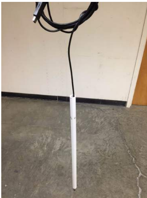
Image 1 (left): Borescope snake camera with pipe casing. At the bottom of the image is where the camera head is held snug with duct tape ring.
