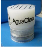
(1) White plastic block with top half of LED light glued on and bottom half of LED light screwed in
