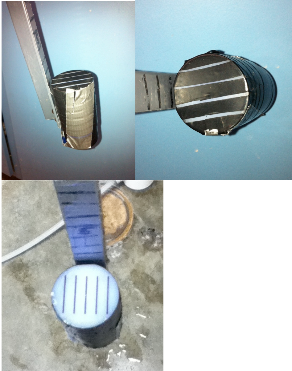
Figure 10: Design for the double HDPE block. First two pictures are of the light slits pattern and the third picture contains the original pattern.
