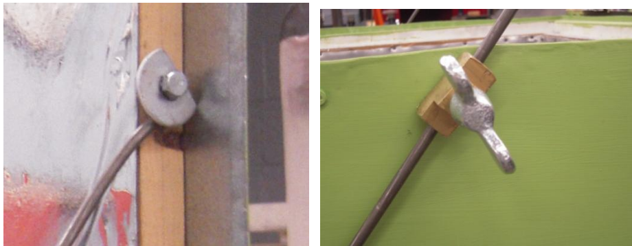
Figure 3: Close-up views of the loop-end of the prop rod and the tee-end of the prop rod
