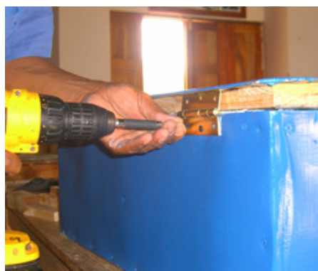
b. Screw in the hinges using 1 ½" screws.
