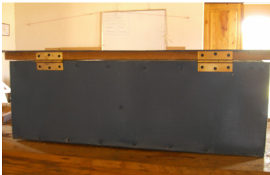
c. Reflector attached to the solar cooker, showing the hinge locations.
