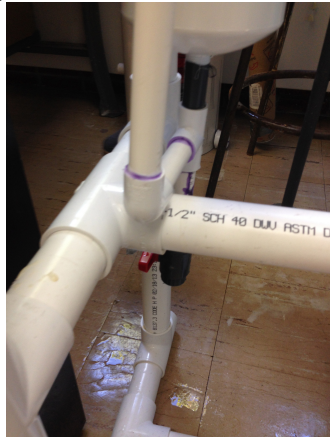
Figure 4: Structure leaking from multiple points throughout experiment Foam Compression Tests
