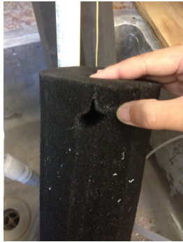
Figure 2: 30 ppi foam without handle after 197 cycles at 200 NTU
