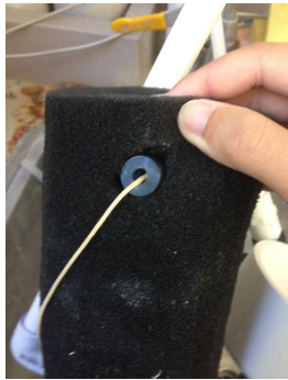
Figure 3: 30 ppi foam with handle after 197 cycles at 200 NTU
