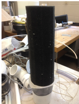
Figure 1: 30 ppi foam after 197 cycles at 200 NTU, noticeable PVC debris
