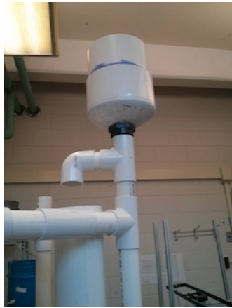
Figure 7: Top of Stand. On the top of the stand, the entrance tank is connected to the leg holding the roughing filter.
