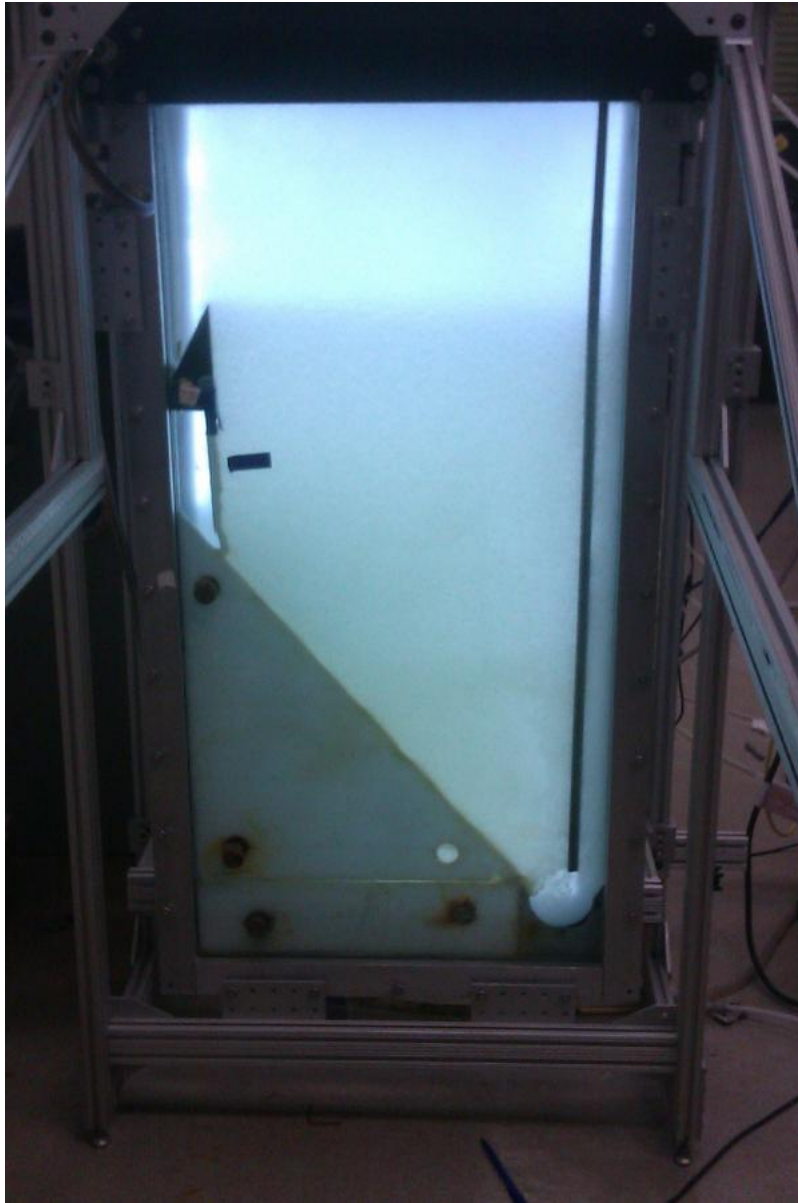
Figure 3: Revised Sedimentation Tank with working Floc Blanket
