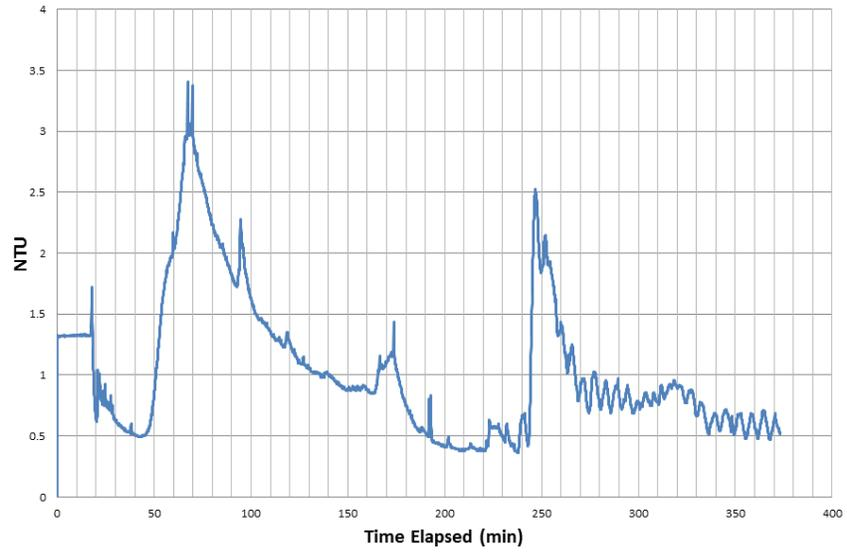
Figure 8: Tube settler turbidity.
