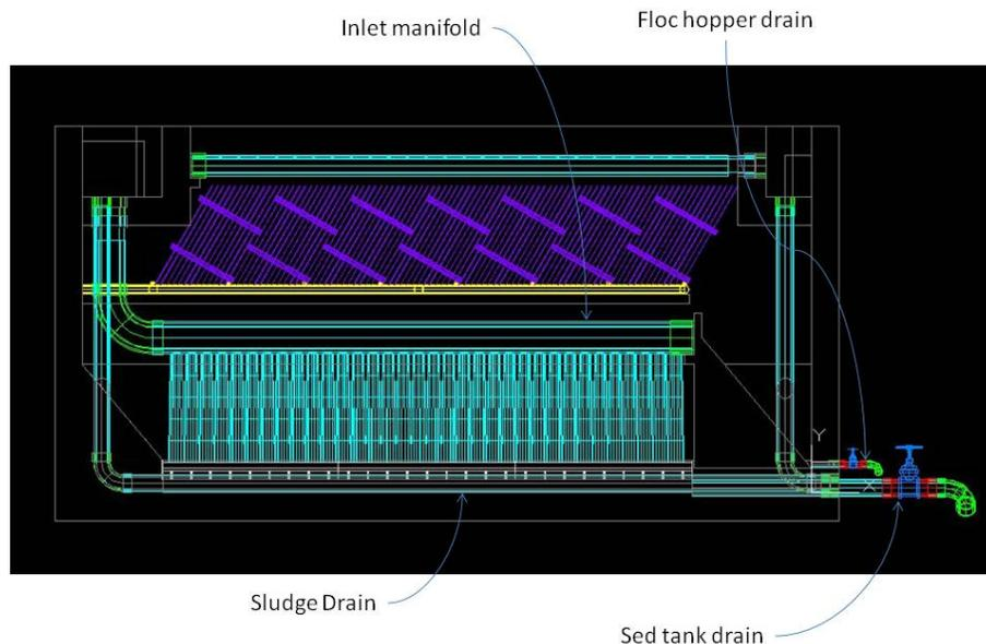
Figure 1: Side view of a typical sedimentation tank
