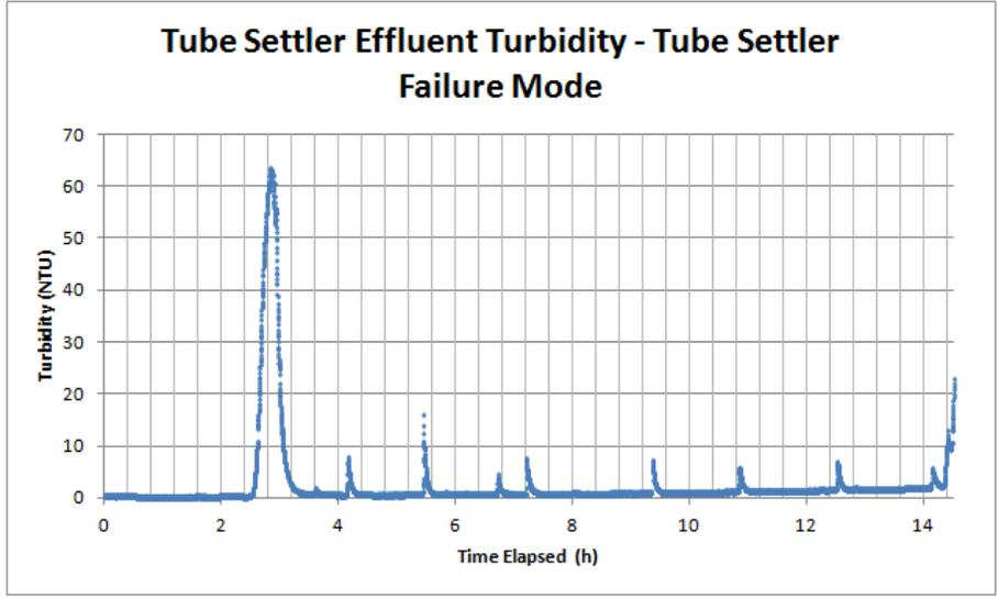
Figure 19: Tube Settler Failure Mode - tube settler turbidity
