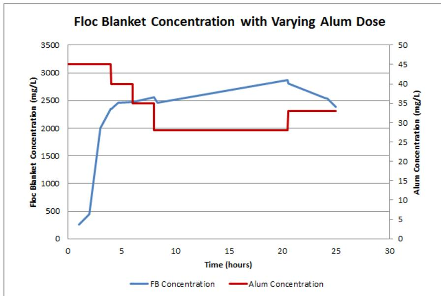
Figure 27: Change in floc blanket concentration with varying alum dose
