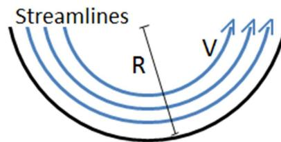
Figure 2: Application of the dynamic pressure equation across streamlines
