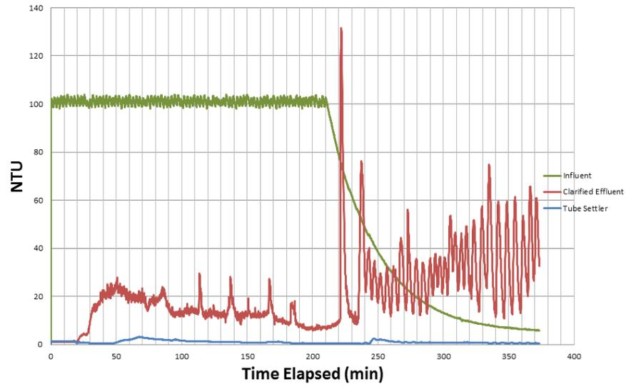
Figure 7: Influent, clarified effluent, and tube settler turbidity
