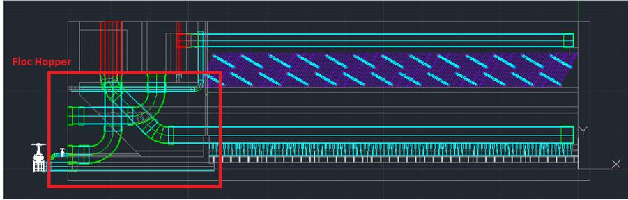
Figure 23: Sedimentation tank with floc hopper (boxed in red) underneath entrance and exit channels
