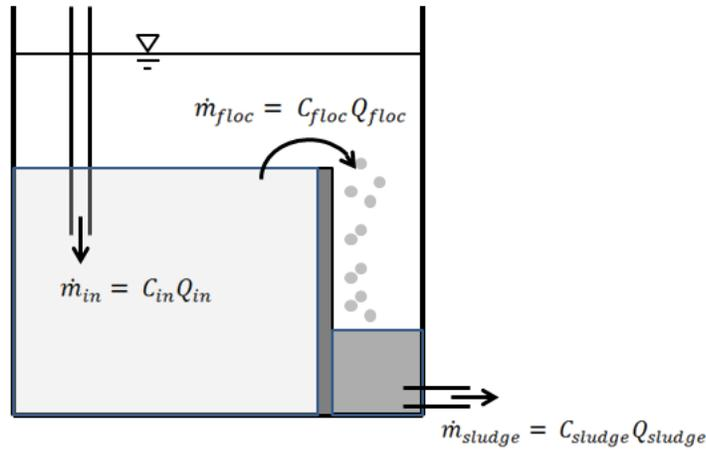
Figure 21: Mass balance of flocculation hopper
