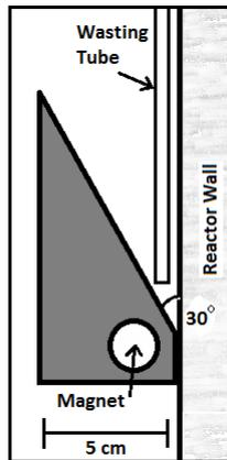
Figure 24: Initial Floc Hopper Design
