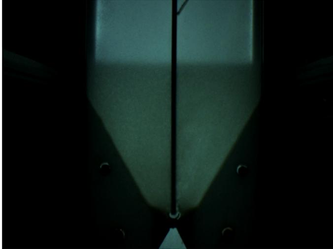
Figure 6: Marcala floc blanket at an influent turbidity of 100 NTU
