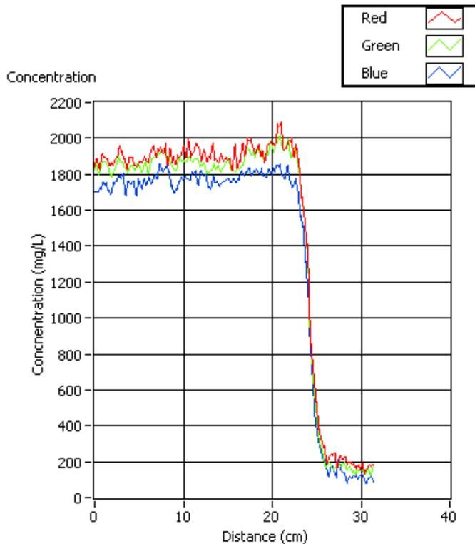
Figure 22: Concentration profile of floc blanket formed with 100 NTU influent. The sharp decline in concentration indicates the location of the floc-water interface.
