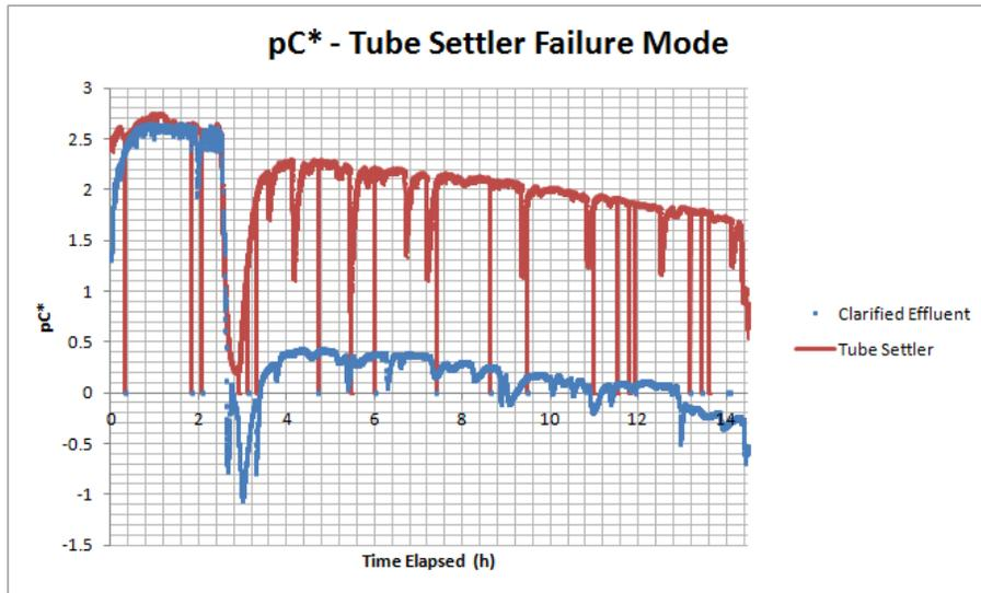
Figure 20: Tube Settler Failure Mode pC\*
