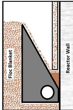
Figure 25: Successful Floc Hopper
