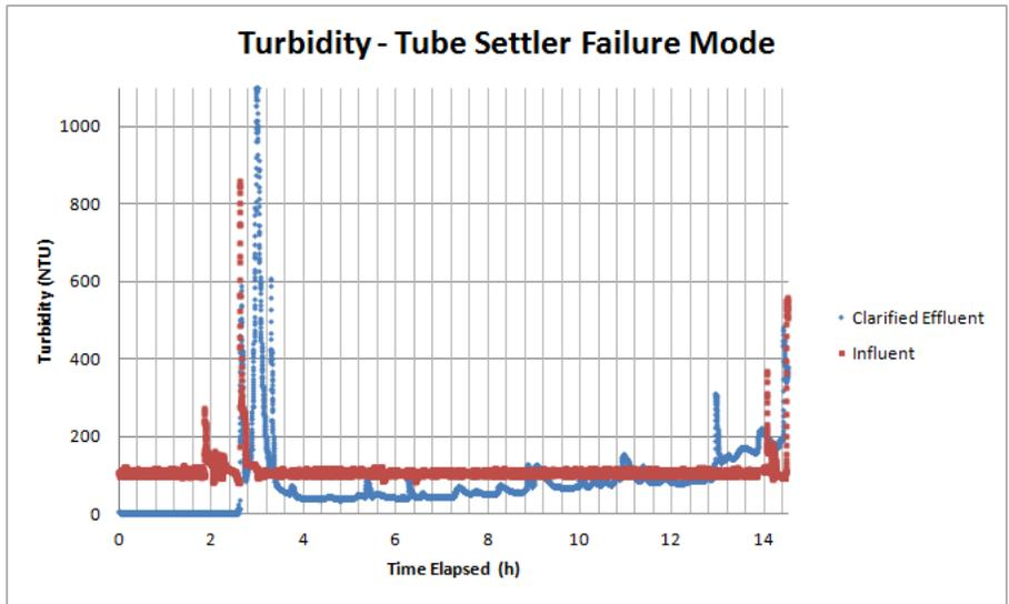
Figure 18: Tube Settler Failure Mode - Influent and clarified effluent turbidity
