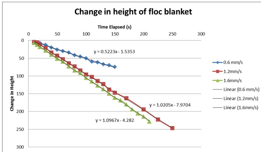
Figure 11: Complete settling curves for upflow velocities of 0.6, 1.2, and 1.6 mm/s
