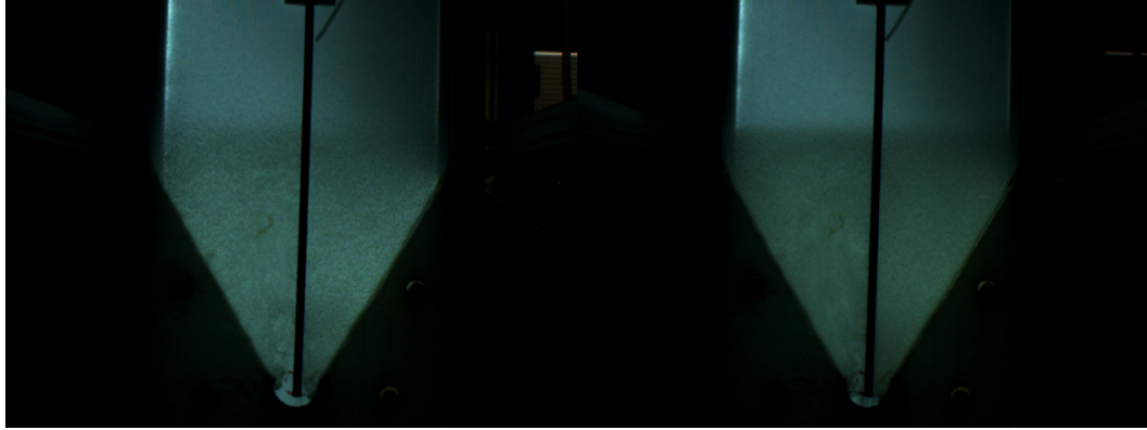
Figure 6: Downward jet displacement at jet flow rates of 556 mL/min and 396 mL/min, respectively.
