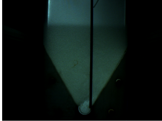
Figure 8: 1.5 inch displacement at inlet jet flow rate of 376 mL/min and upflow velocity of 0.49 mm/s.
