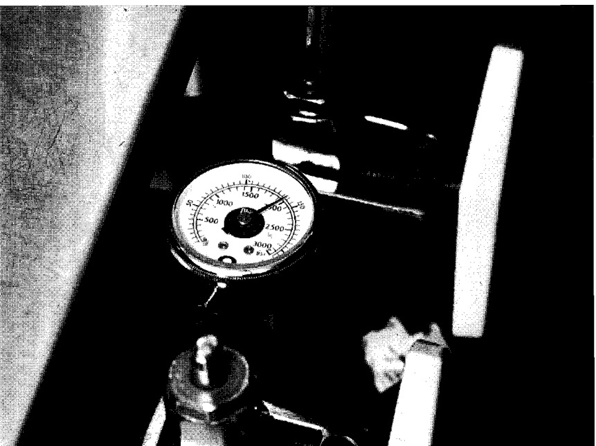
Fig. 17.67. Oxygen cylinder with the pressure gauge reading 2000 psi. An oxygen cylinder should have at least 500 psi before the cylinder and anesthesia machine are used with a patient. With oxygen flowmeters off, the cylinder valve should remain on to allow evaluation of the machine for slow leaks.
