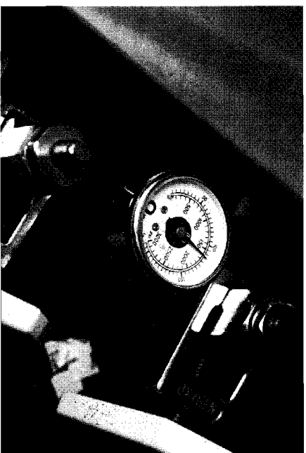
Fig. 17.68. Oxygen cylinder with the pressure gauge reading at 1700 psi after 15 min with the cylinder valve open. If the cylinder pressure was 2000 psi at the start of the test and the flowmeters were off, a significant leak is present and should be corrected before the anesthesia machine is used with a patient.
