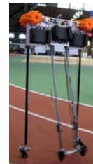
The Cornell Ranger robot walked 5.6 miles on April 3, 2008 powered by a 2 lb Li-Ion battery. The project demonstrates the synergy of theoretical mechanics with practical engineering and the education of our students.
