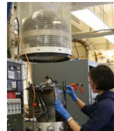
PhD student Sara Barron (van Dover Group) using a vacuum deposition system in the lab
