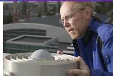
Professor Paul Kintner, shown positioning the antenna on the roof of Phillips Hall, discovered that strong solar flares cause Global Positioning System receivers to fail.
