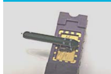
This prototype device uses a copper cantilever 2 centimeters long. Future nanofabricated versions could be smaller than one cubic millimeter; created in Assistant Professor Amit Lal's lab.
