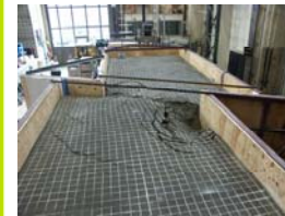
Simulation of an earthquake for lifeline testing in the CEE laboratory.
