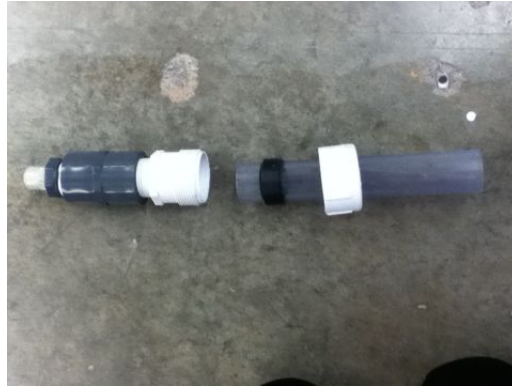
Figure 12: Attaching Sedimentation Tank Fittings
