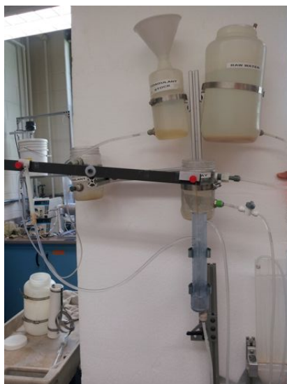
Figure 3: Stock Arm and Doser Close-Up
