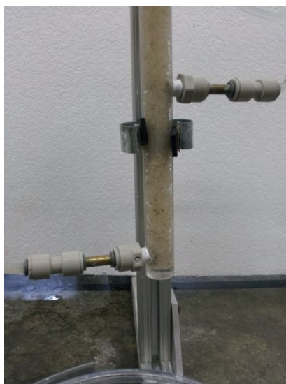
Figure 17: Example Location of Filter Fittings Relative to Broomhandle
