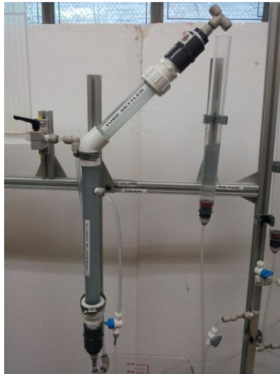
Figure 11: Sedimentation Tank and Drop Tube
