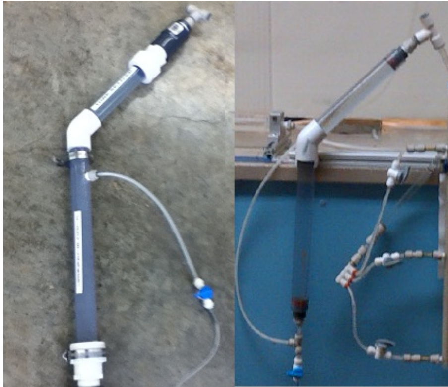
Figure 12: Old and New Sedimentation Tanks
