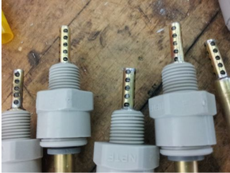
Figure 3: Compressed springs in inlet and outlet pipes
