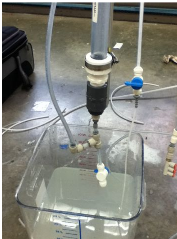
Figure 8: Emergency Floc Drain
