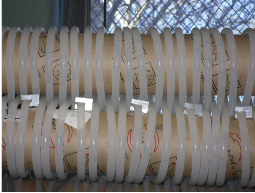
Figure 9: New floc breakup devices (aluminum pieces)
