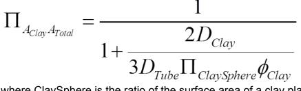
where ClaySphere is the ratio of the surface area of a clay platelet to the surface area of a sphere of equivalent volume. AClayATotal is the ratio of the clay surface area in the flocculator to the total area of the flocculator walls plus clay.
