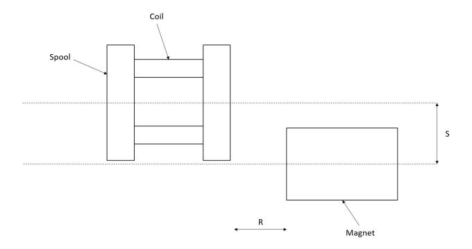
In the first case, the current will vary from 0-100mA in 10mA intervals. In case two, the axial displacement will vary from 0.0-.5mm in 0.05mm intervals.
