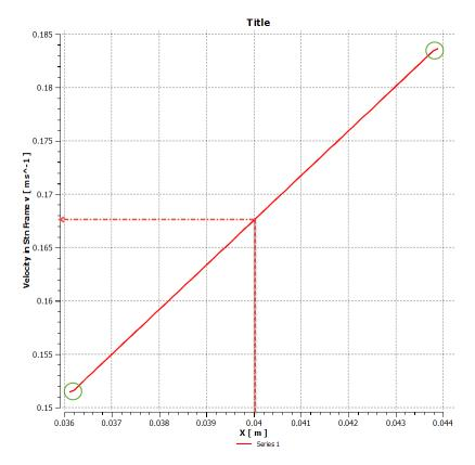
The point is slightly above the halfway between 0.165 and 0.170. Recall from pre-analysis that we calculated the expected value as 0.1676m/s. The value is virtually the same, indicating that we might have inputted the right mathematical model into the tool.
