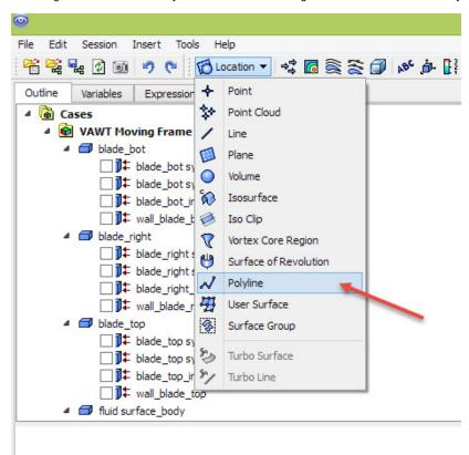
Name it "wall right" and for "Method" select "Boundary Intersection". For "Boundary List" select "blade\_right symmetry 1" and for "Intersection With", select "wall\_blade\_right". Click Apply.
