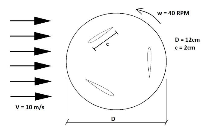
Consider a uniform flow of V = 10m/s passing through a Vertical Axis Wind Turbine (VAWT) as sketched above. The VAWT has a diameter of 12cm and 3 equally spaced blades, each one with a chord length of 2cm. For simplification, consider that it spins with a constant angular velocity of 40 RPM\*. The center of each blade is located 0.04m from the center of the hub.
