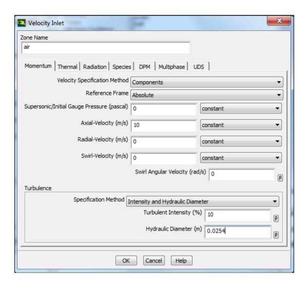
Similarly, edit the air-fuel boundary to have velocity components, with 50m/s axial velocity and 30m/s swirl velocity. The turbulent intensity should be 10%, but the hydraulic diameter should again be 0.0254m. Clicking to the Species tab, change the mean mixture fraction to 1.0. This is because this stream will be taken as the fuel stream, whereas the previous air boundary did not need to be set beyond the default value of 0 for the oxidizer stream. Click "Ok".
