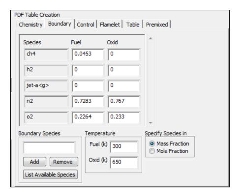
Ignore the Control and Flamelet tabs, and select the Table tab. Click "Calculate PDF Table" to generate the pre-computed PDF table denoting mixture fractions that will handle the non-premixed combustion analysis. Investigate PDF table parameters and dependencies by clicking on "Display PDF Table", selecting desired options, and clicking "Display.
