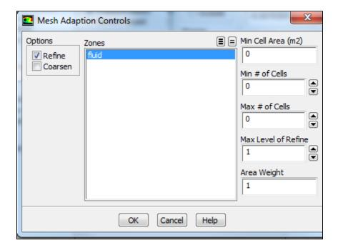
Then, click Select Points with Mouse. Select the probe button to enable point selection and right-click with your mouse just below the bottom left corner and just above the top right corner of the mesh so that the entire mesh is selected for grid adaption.
