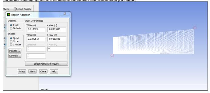
Finally, click Adapt. Display your newly adapted mesh: Solution Setup - General; click on "Display" and select "fluid" as the surface. Press Display again, and then close the dialogue. The mesh should now look like this:
