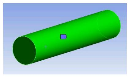
With **Boundary** highlighted, select the lateral surface using face selection tool,
